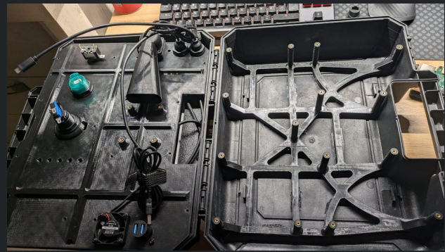
Figure 5. GCS being assembled on a tools box
